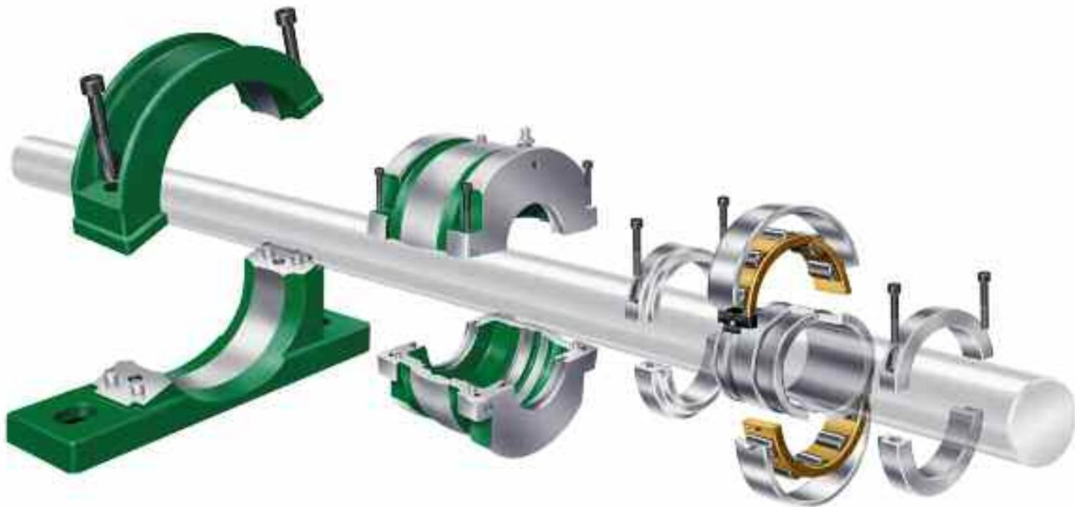
**Bearings** are effectively the messenger of rotating equipment in that they support the load rotating. Often there is a problem with the rotating load which impacts on the bearing, these problems will be reflected in heat and or increased vibration and may be indicated or diagnosed by observing abnormal wear patterns.
